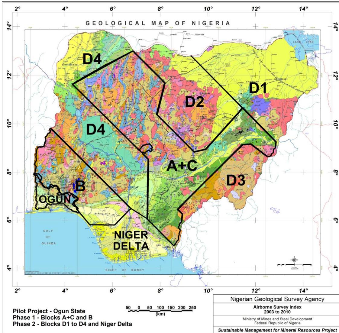
Figure 1: Index map of the airborne survey blocks flown between 2003 and 2010 for the Nigerian Geological Survey Agency (electromagnetic surveys not shown). In the background is the Geological Map of Nigeria (NGSA, 2006).
