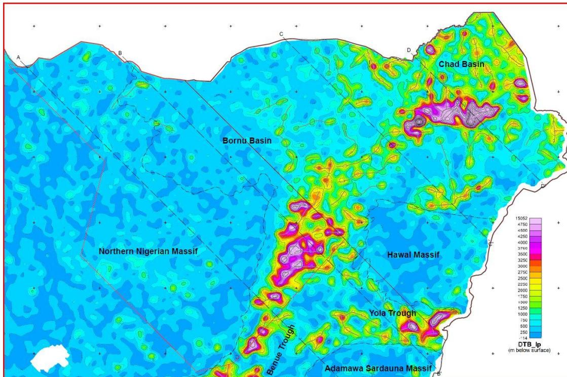
Figure 2: Depth-to-magnetic source map for northeast Nigeria.
