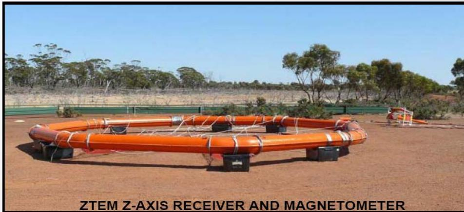
ZTEM Z-AXIS RECEIVER AND MAGNETOMETER
