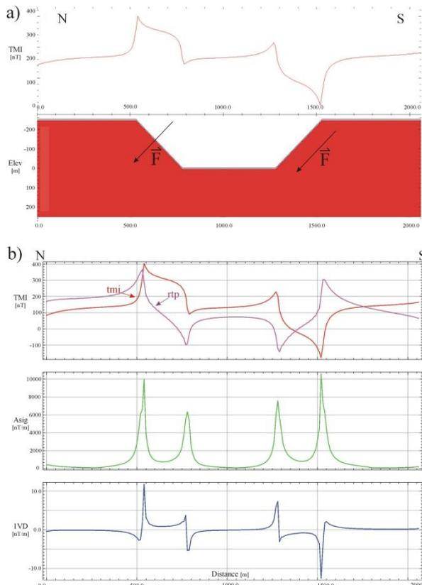
Figure 1: synthetic model of a magnetized valley under an inclined effective magnetic vector. The block has uniform susceptibility of 0.01 SI and observation level is 2 m above the ground, simulating a ground survey. Top panel shows TMI and RTP profiles; middle: amplitude of the analytic signal from the TMI; bottom: first vertical derivative of the TMI.
