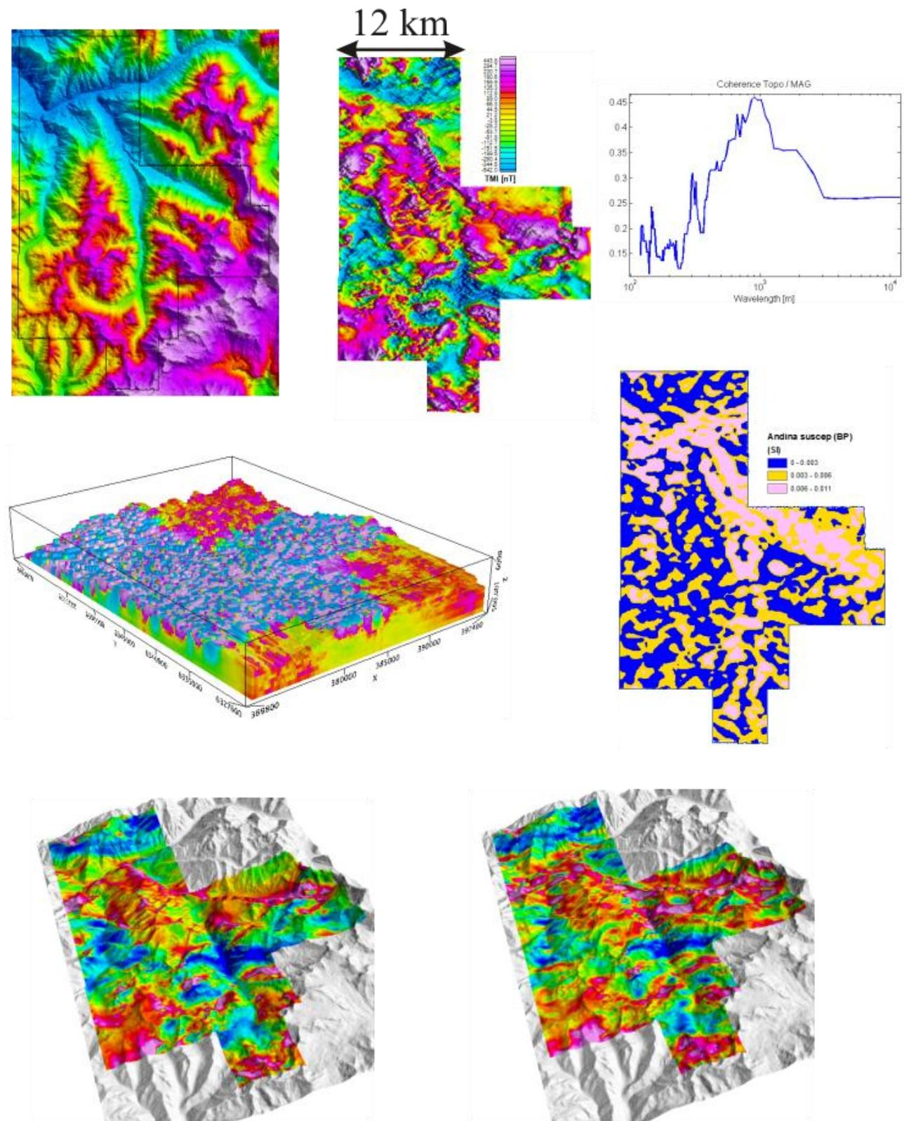
Figure 2: Application of the topographic correction algorithm to a case in the Southern Andes. Top left: SRTM topography (blue = 1500 m; purple = 5200 m); top-middle: observed TMI data; top-right: coherency between both signals. Middle-left: 3D inversion of the band-passed data based on the coherency analysis; middle-right: susceptibility model derived from the 3D inversion. Bottom-left: uncorrected TMI draped over the topography; bottom-right: final corrected TMI data.
