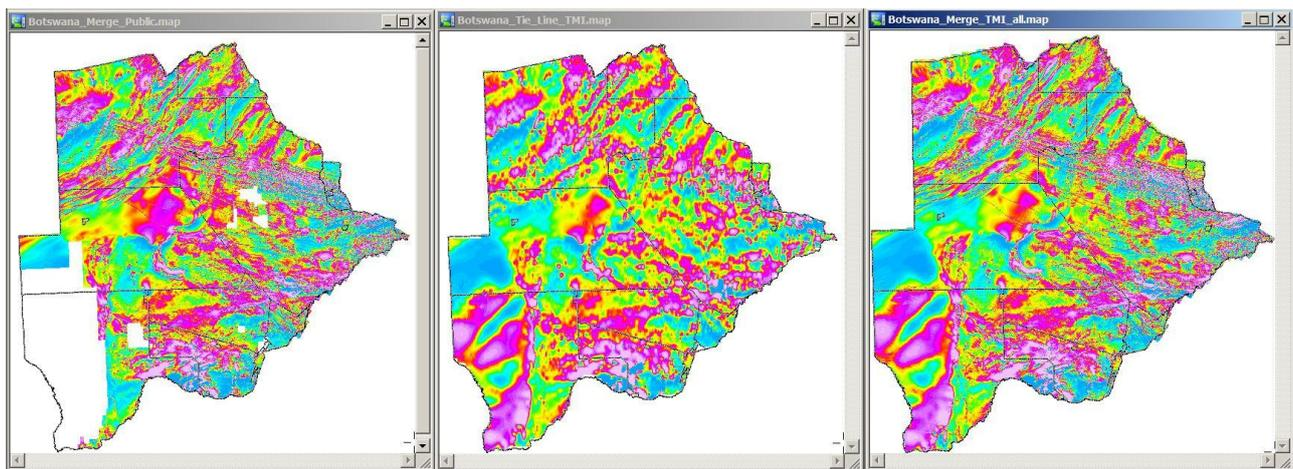
**Figure 4. Comparison of previous and new nationwide total magnetic intensity (TMI) merge: Left – Previous merged TMI, Centre – Tie line survey TMI, Right – New merged TMI.**
