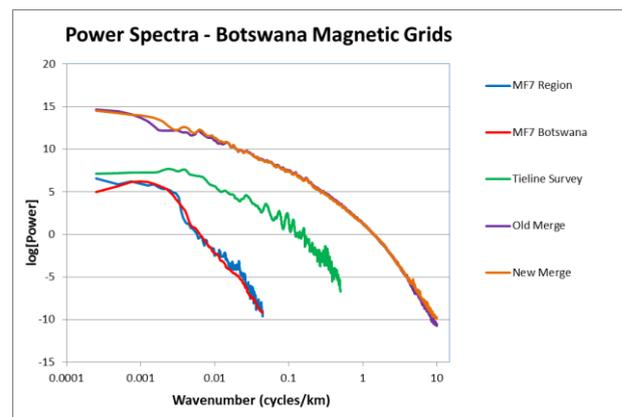
**Figure 5. Comparison of power spectra for TMI grids of satellite magnetic data (CHAMP model MF7), the Tie Line Survey, and previous and new merges.**
