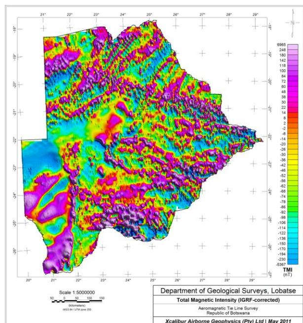
Figure 2. Total magnetic intensity after IGRF correction for the Botswana Tie Line Survey.
