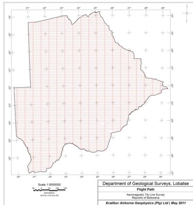
Figure 1. Flight path for Botswana Tie Line Survey.
