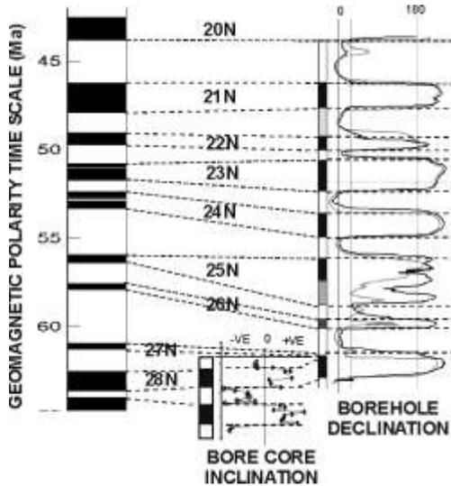
Figure 5 Comparison of magnetic reversal stratigraphic record as interpreted from borehole magnetic log of UNAM-7 and reference Geomagnetic Polarity Time Scale. Results of paleomagnetic study of core samples from UNAM-7 are used to establish reference point for matching borehole and reference polarity scales.
