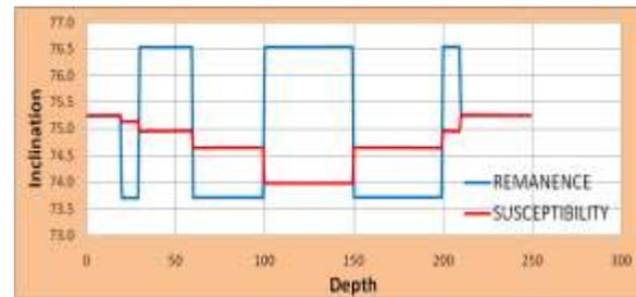
Figure 3 Diagram to show the effect of increasing magnetic susceptibility and alternating normal and reversed polarity remanence on the observed magnetic vector.
