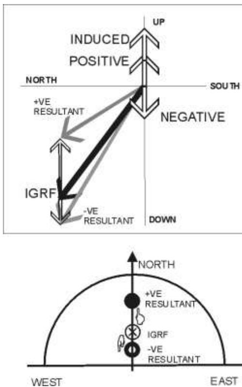
Figure 2 a) Diagrammatic representation of vector summation of induced and remanently magnetized crustal field components with
