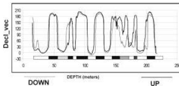
Figure 4 Plot of declination change versus depth for up and down hole logs from borehole UNAM-7. Up-hole survey was acquired at half the speed used in the down-hole survey.
